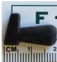
Figure 7: 3D-printed leg of Tango Plus FLX930 with a shore hardness of 27.
